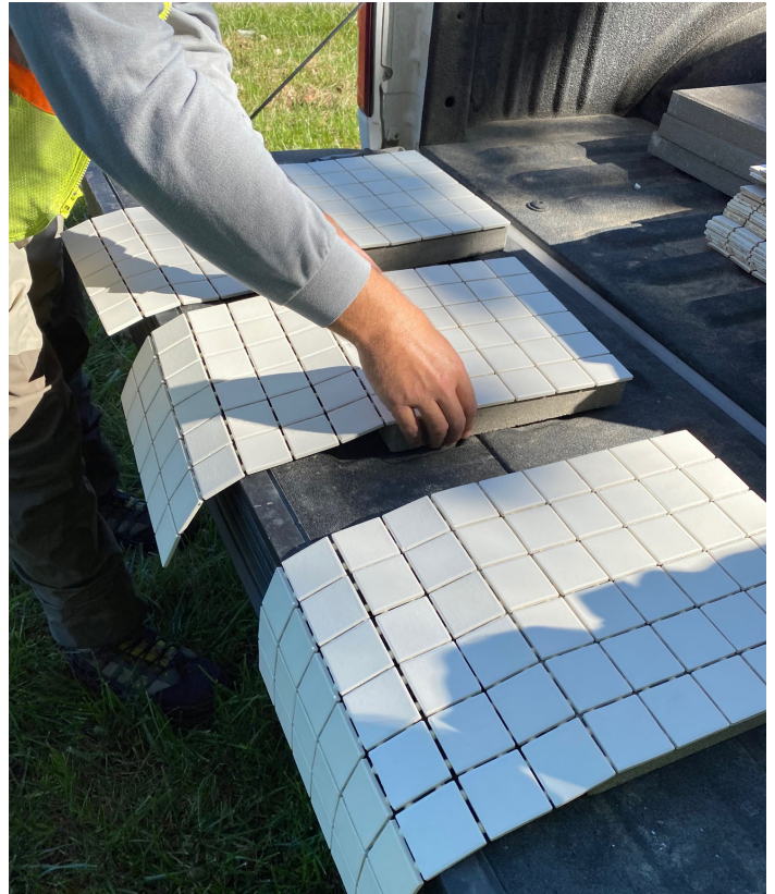
Half a dozen 6- by 12-inch sheets of 1-inch tile squares are left in place in the waterway for about 16 days in the fall, allowing algae to grow on the tiles.
