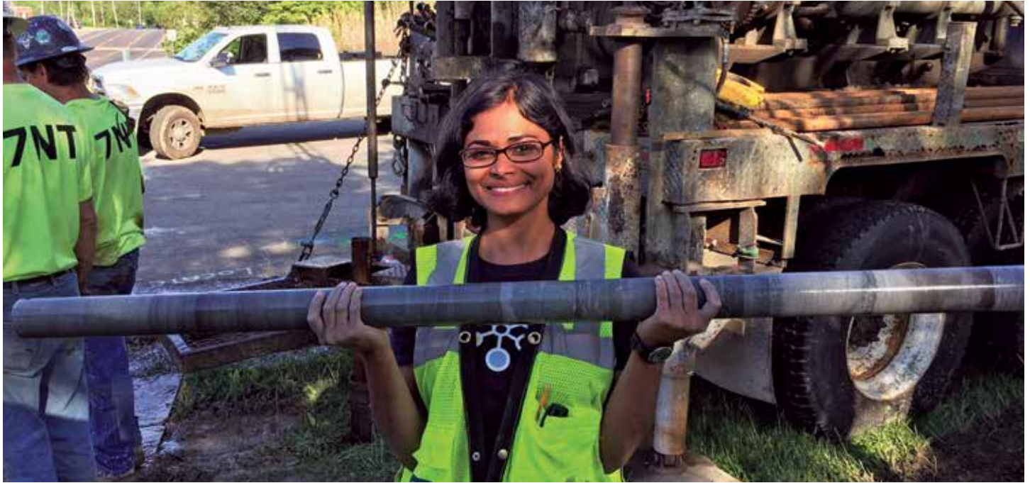
Rock core samples were used to determine the depth necessary for safe construction of MSD's Waterway Protection Tunnel.
